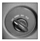
If your vehicle is equipped with four-wheel drive, the transfer case knob is located to the right of the steering wheel on the instrument panel. Use this knob to shift into and out of four-wheel drive.
